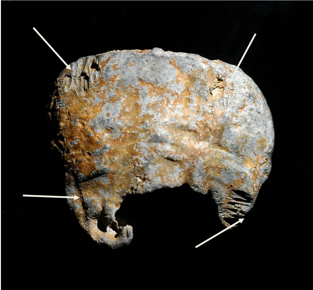
Figure V:27. Flintlock Jaw Marks
